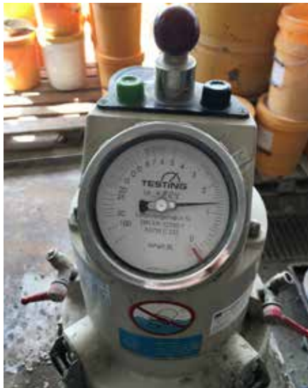
Figure 4.2.4.1: Air meter (ASTM C 231 - Type B) for air content test
