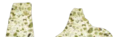
Figure 1.1.3: Forms of slump
