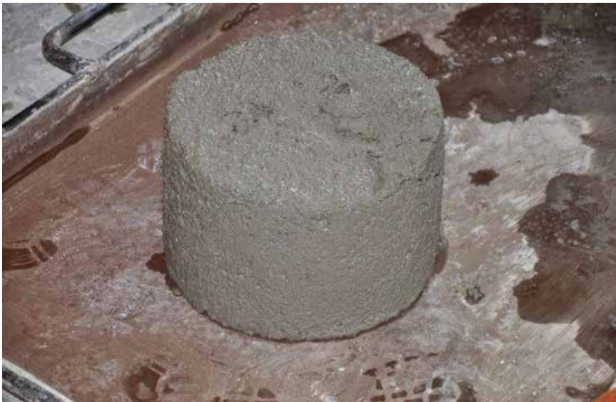
Figure 4.2.1.4: RCC sample after consolidation with Vebe apparatus
