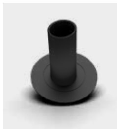
EPDM rubber roof outlet , applied by torch method and compatible with any type of bituminous membrane. With different heights and diameters.
